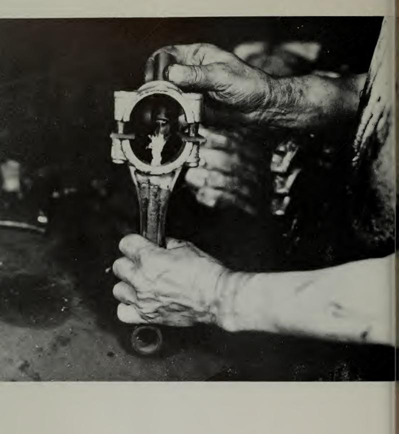
Any oil holes appearing in various places on the cap or the bearing end of the rod (varying with the type of rod) are plugged with asbestos wicking as shown above. In some instances small cork stoppers are used and even toothpicks on the smaller rods. This caulking process prevents the babbitt from plugging up the oil holes.
